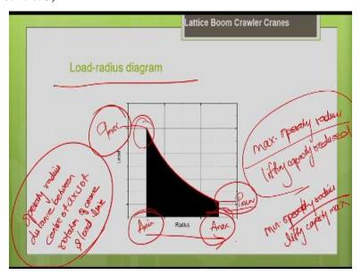
So, after determining the load L, you can plot this load radius diagram as shown in this picture, you can see. As the radius increases as the operating radius increases, so, what is happening to the
