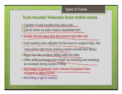
So, now, let me summarize. The truck mounted telescopic boom, mobile crane, they are capable of quick traveling from side to side. Mobilization is very easy; can be driven on public roads in assembled form. It greatly reduces the setup time and cost but high initial cost that you have to note it. So, if job requires crane utilization for few hours to couple of days, this crane will be the right choice.
