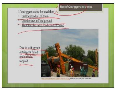
As I told you, use of outriggers is very important when you go for tire mounted cranes that is very important for the stability of your crane. So, without outriggers, you cannot get your desired lifting capacity. So, you can see this picture where the crane is toppled so, because of the poor soil conditions. So, before planning the use of crane, you have to check for the soil conditions.
