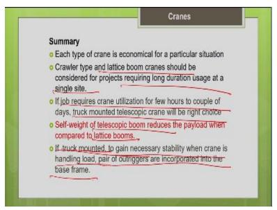
So, the lattice boom crane, it will be economical provided you need the crane for a longer duration of the single project site. In that case, it will be economical. If you need it just for a few hours, it will not be economical because its mobilization cost, erection-dismantling cost is going to be higher. So, if you need it for a longer duration, go for the choice of lattice boom cranes and crawler type cranes.
