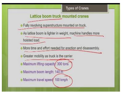
So, basically the lattice boom truck mounted crane as the revolving superstructure mounted on truck. Here also, since it is lattice boom, we get the advantage. Boom is lighter in weight. So, the machine can handle more hoisted load. The demerit is, the erection and dismantling take more
