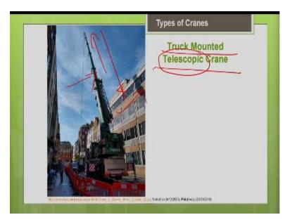
So, we have discussed about the lattice boom crawler crane, lattice boom truck mounted crane. Now, we are going to see telescopic boom cranes, truck mounted telescopic boom crane. So, as the name indicates just like a telescope, you can extend the length of the boom or retract the length of the boom. Just this is the boom. You can see, this is a telescopic boom. You can extend the length of the boom or retract the length of the boom depending upon your working range requirement.
