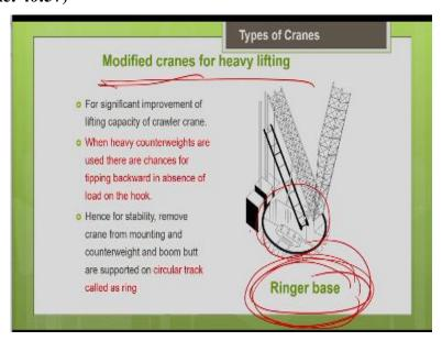
So, another important type of crane is modified cranes particularly for heavy lifting applications. Say for example, if I need a lifting capacity of 1000 tons, 2000 tons, these are very rare cases,
