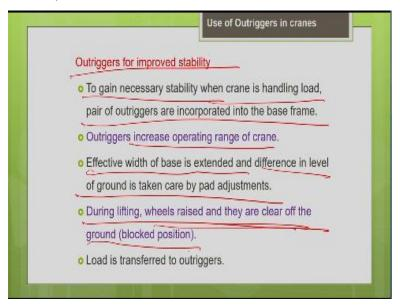
So, let us see what is the main purpose of going off for outriggers. So, outrigger is mainly intended for improved stability of your crane. To gain necessary stability when the crane is handling the load, pair of outriggers are incorporated into the base frame. They increase the operating range of the crane. They widen the base area. So, that you can have a better lifting capacity.
